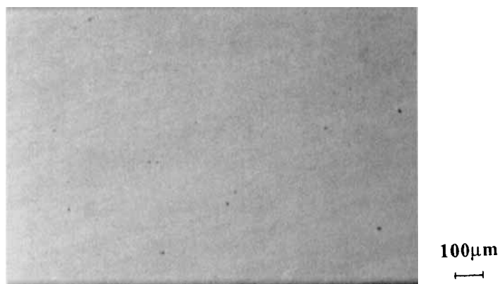
Figure 8. A microphotograph showing the alignment of the ferroelectric liquid crystal cell containing compound 2. The photograph was taken under dark-field illumination and using crossed polarizers (magnification \times 40 ).
